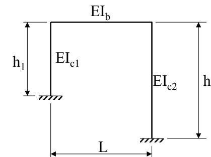
1.2 For the special case of  $I_{c1} = I_{c2} = I_b$ ,  $h_1 = h_2 = h$  and  $L = 2h$ , find lateral stiffness  $k$  of the frame.
