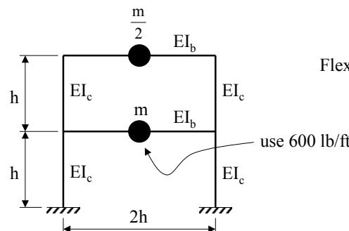
Flexural rigidity of beams and columns
